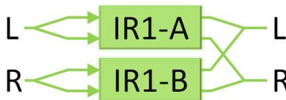
3. Mono to Stereo: The left and right input channels are mixed to mono and then independently convolved with the left and right impulse response file channels. When using a single stereo impulse response file, this is useful when input audio is panned hard left or right; this configuration is often encountered in low/medium-end stereo algorithmic reverbs.
